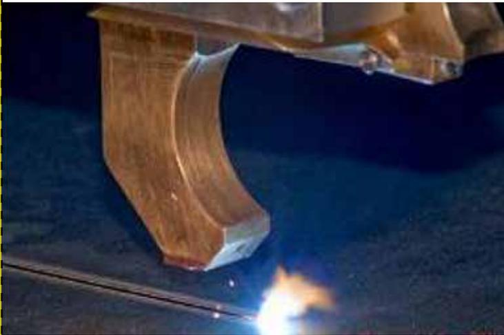
*The LASAL Jet Nozzle argon gas dynamic yields effective plasma suppression with more efficient and wider shielding coverage.*
