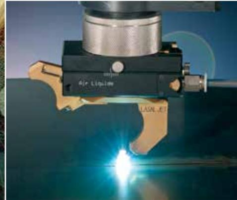
The high performance **LASAL Jet Nozzle** for Laser welding solution features a unique jet nozzle designed to enhance gas shielding effectiveness and plasma suppression. It yields excellent CO<sub>2</sub> laser welding quality and speed when totally **replacing helium** with argon gas, with no need for additional gases and a mixer. The net result is enhanced performance, with minimized welding defects scrap rates while considerably reducing operating costs.
